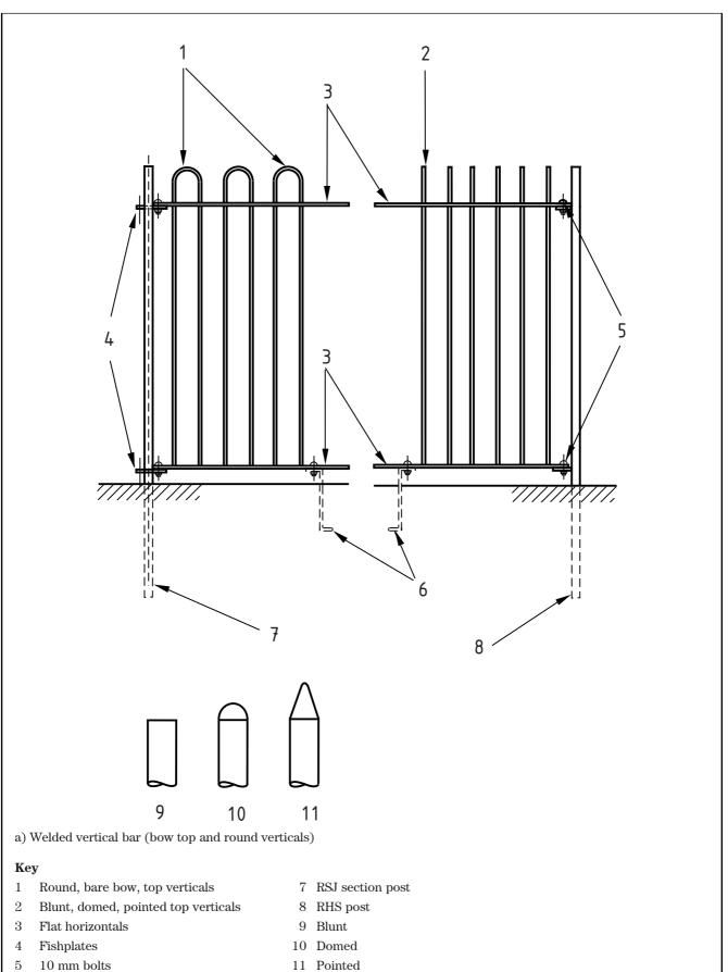
Figure 1 Typical fence with round and square verticals and flat horizontals (continued)
