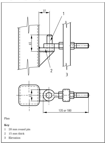
Figure 2 Examples of typical hinge profiles (continued)
